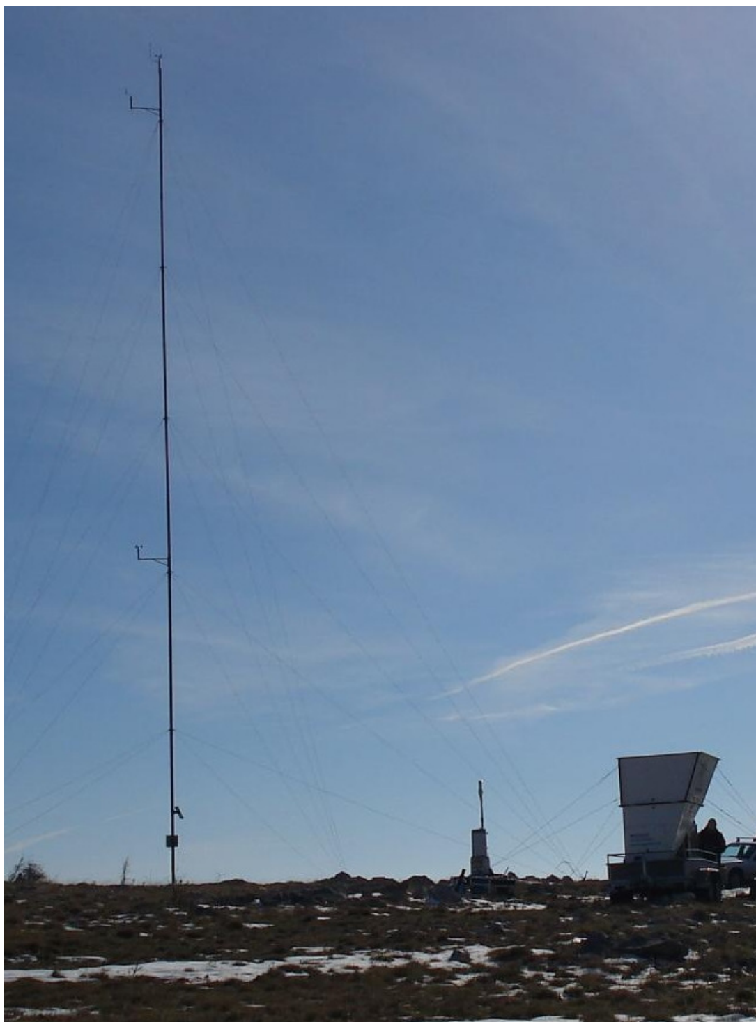
Fig. 3: Picture with the 30 m mast (right), the LIDAR (middle) and the SODAR (left).
