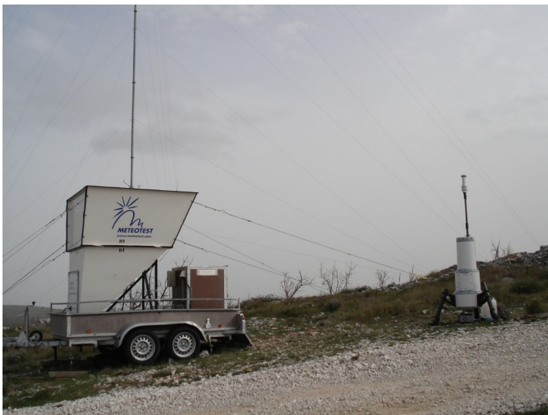
Fig. 3: Picture with the SODAR (left), the LIDAR (right) and the 50 m mast in the background facing southeast.
